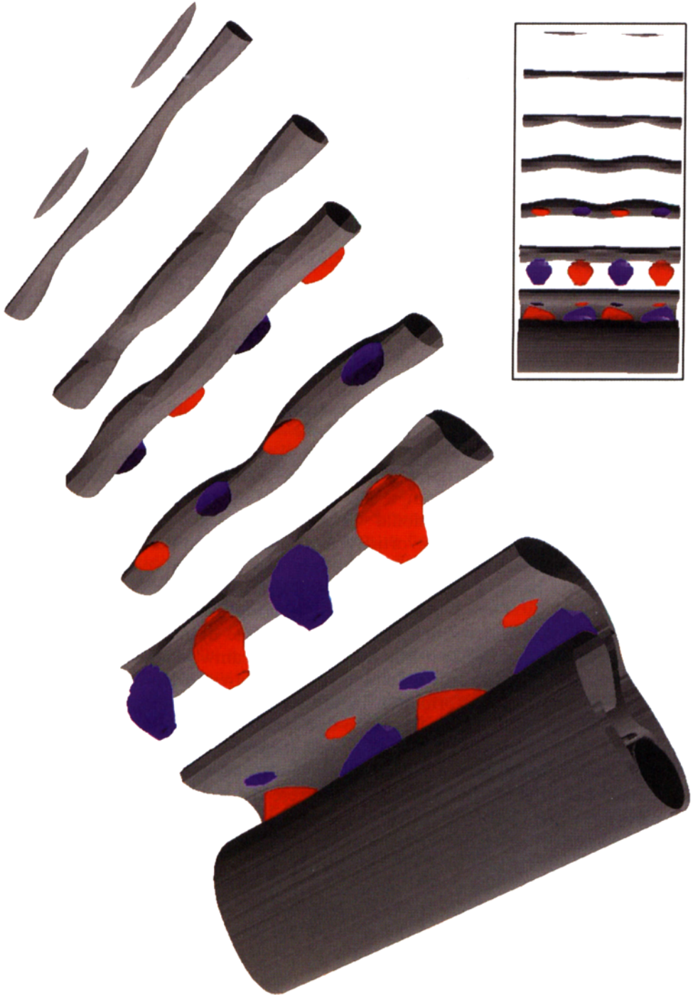
FIGURE 9. Superposition of the critical Floquet mode on the von Kármán vortex street. The grey tubes are isocontours of spanwise vorticity magnitude, |\zeta_z + \hat{\zeta}_z| . The critical Floquet mode gives rise to a spanwise-periodic deformation of the primary von Kármán vortices. Linking these vortices are thin regions of positive (red) and negative (blue) streamwise vorticity, \hat{\zeta}_x . The inset shows a view of the same structure from above. Data for this figure were taken from image (a) of figure 10.
