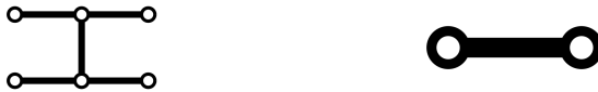
Figure 2.6: Illustration of the RG approach to the 2D bond percolation where the black lines and empty circles represent bonds and lattice sites, respectively. A five-bond RG unit (Left) is mapped onto a single super bond (Right).
